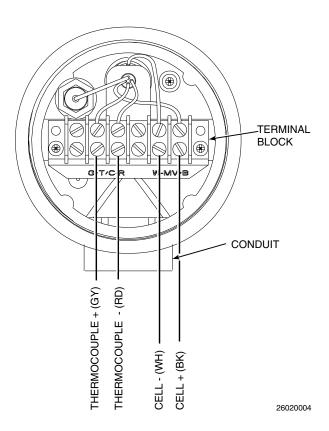
Figure 2-9. Oxygen Probe Terminal Block
